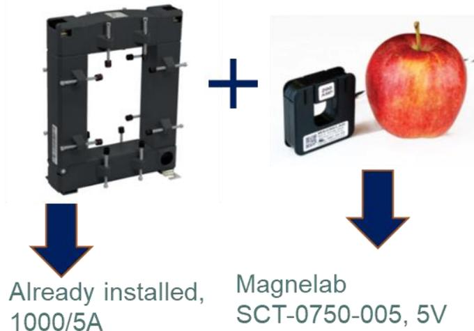
**Figure 25: Combination of current transformers for SMU installation (left; existing 1000/5A, right: new current sensor connected to SMU).**
