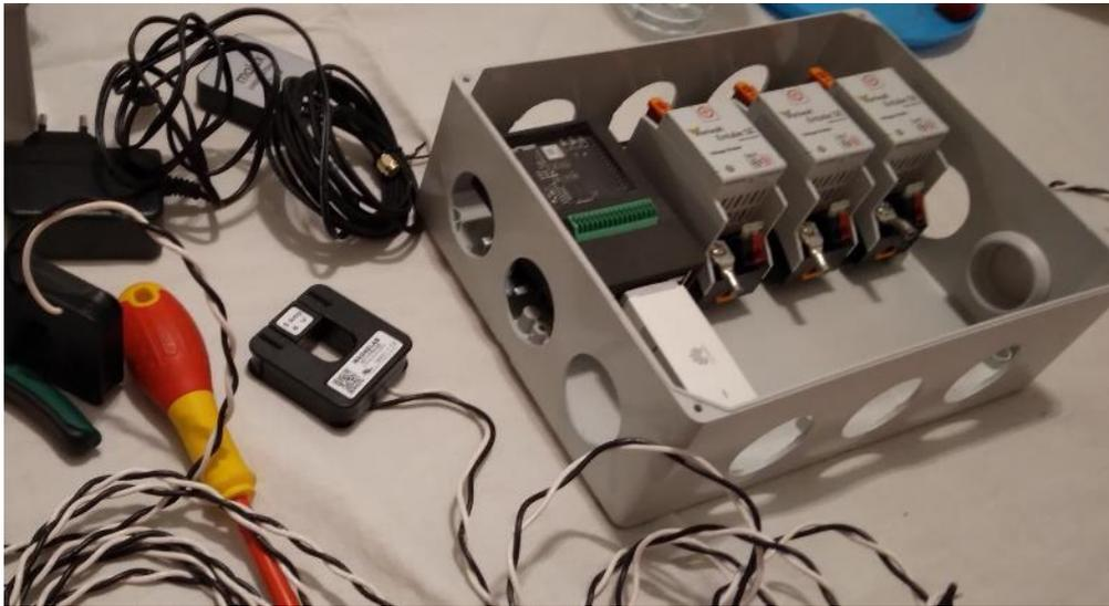
Figure 28: Assembly of SMU and sensors in the box.
