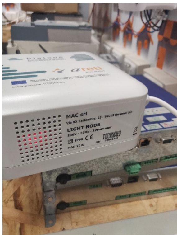
Figure 16 Light Node and smart meter in areti's lab
